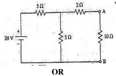
b) Find the value of  $R_L$  for the given network below so that the power drawn by  $R_L$  is maximum.
