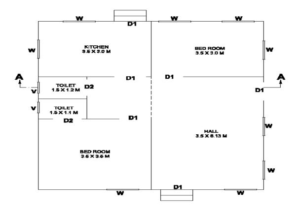
2. The line sketch given below shows the plan of a residential building. The dimensions given in the sketch are internal dimensions of the rooms. Draw the Cross section along ABCD of the given line sketch to a scale of 1:100
